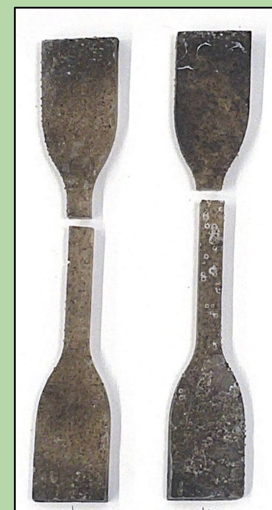
Figure 3b: Breakage points of the 1% coffee dog bones
