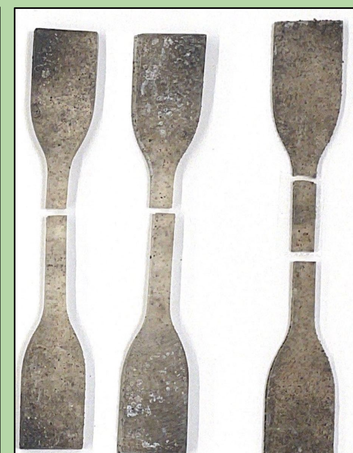
Figure 2b: Breakage points of the 0.5% coffee dog bones
