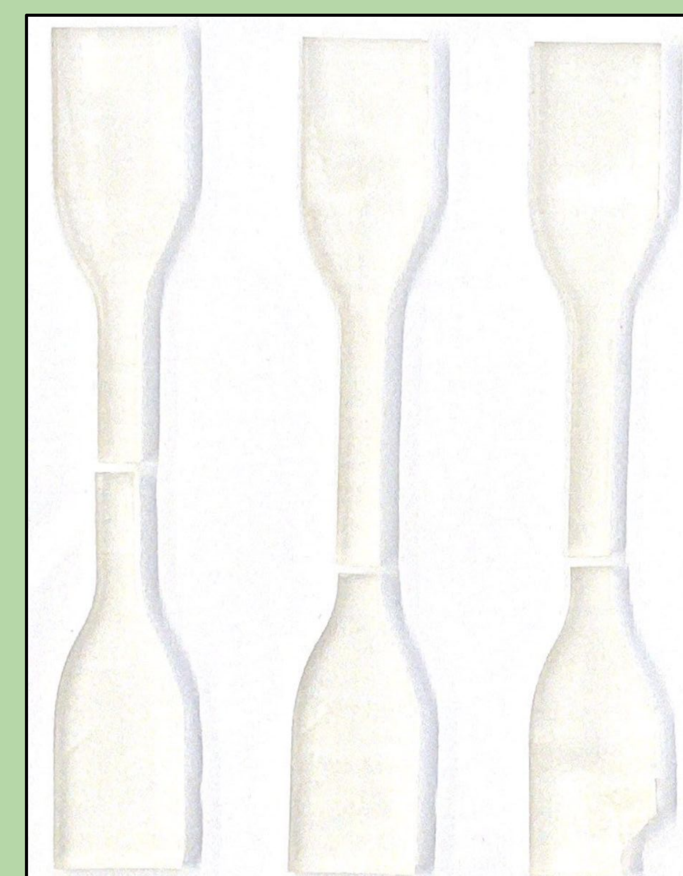
Figure 1b: Breakage points of the clear dog bones
